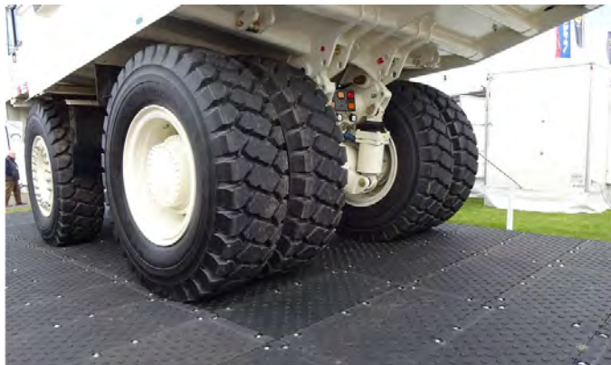
Mats can be locked together to form a workable platform.
